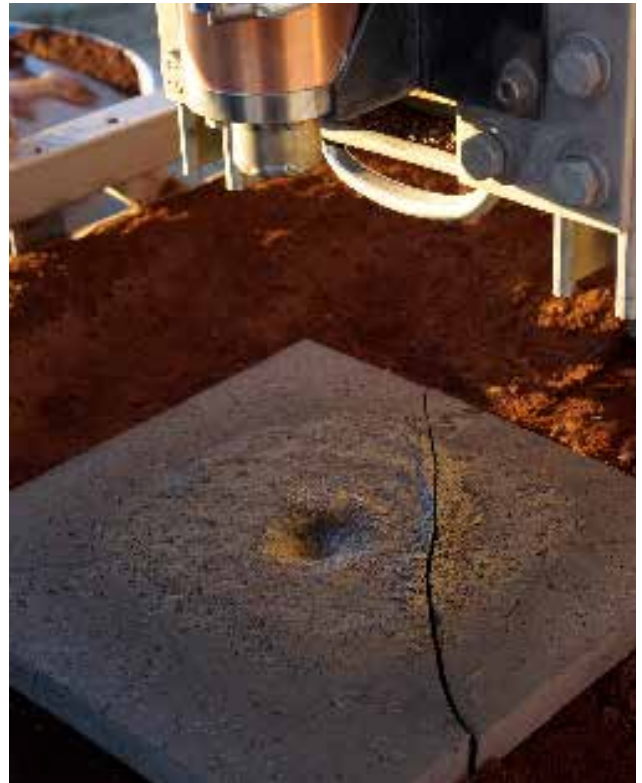
Above: A 12" x 12" sintered basalt tile created at PISCES was tested as a launchpad material last month. Photo: Masten Space Systems.
