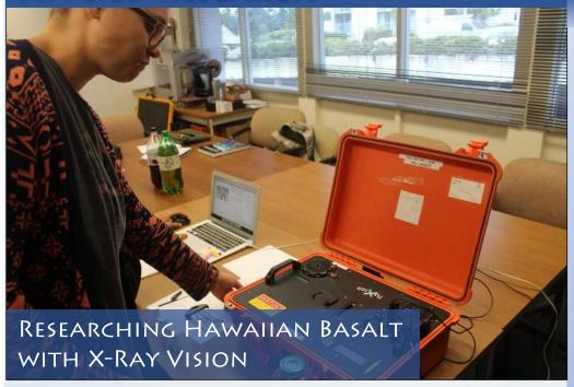
PISCES Geology Tech Kyla Defore prepares Hawaiian basalt samples for X-ray analysis.
