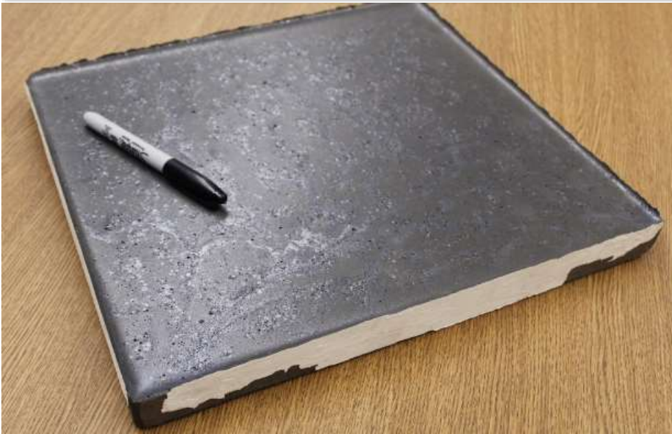
Above: A sintered basalt tile measuring 13" x 13" x 1.5" is the largest basalt product created by PISCES so far. The 15-lb. block was made using no additives—just basalt and heat.
