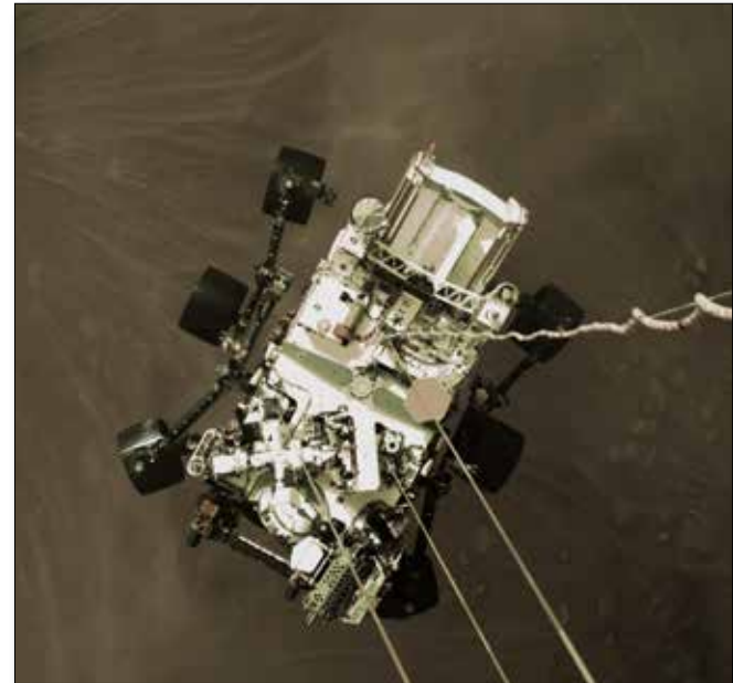
Above: NASA's Perseverance rover is lowered to the Martian surface from a jet-powered sky-crane on Feb. 18. Image credit: NASA-JPL.
