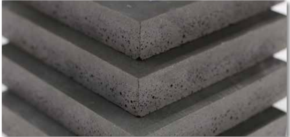
Above: Sintered basalt tiles made with a binding agent are structurally comparable with the previous generation of tiles (shown above).
