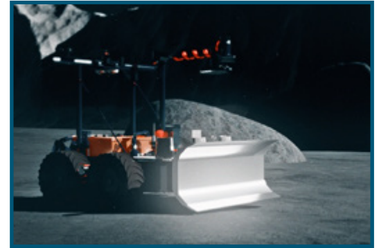
Above: Artist rendering of a lunar rover equipped with a leveling blade for excavating the surface of the moon. Credit:
