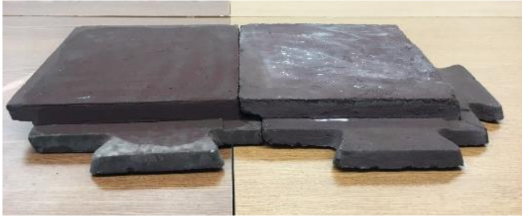
Figure 4: Interlocking Pavers made with sintered basalt used in the construction of a landing pad in Hilo, Hawai'i.
